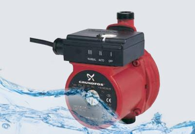
The UPA Homebooster is a circulator pump designed for pressure boosting hot water systems. The pump provides additional pressure to showers, taps and similar outlet points. The UPA Homebooster is for use in open systems. The pump incorporates a flow switch which starts or stops the pump when a tap is turned on or off.
